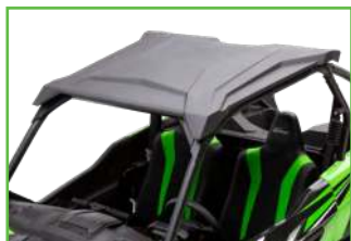
KQR Plastic Roof (Injection Molded)
